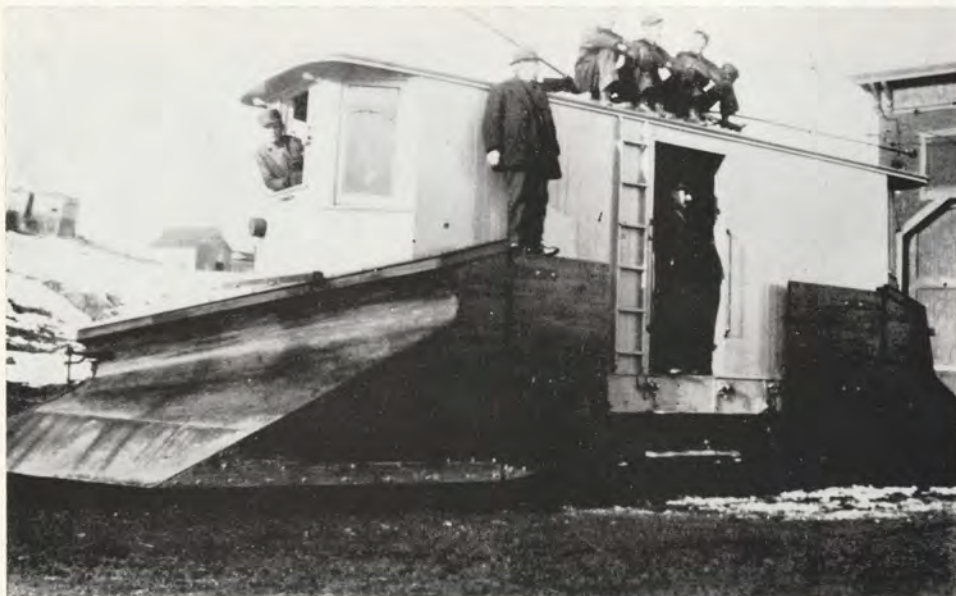
PLOW NO. 2 at the Fairfield carhouse about 1904. It was built about 1900 by the Waterville & Fairfield Railway and it is said the plow blades were fabricated at the Maine Central Railroad shops in Waterville. —[Lloyd A. McAuley.
