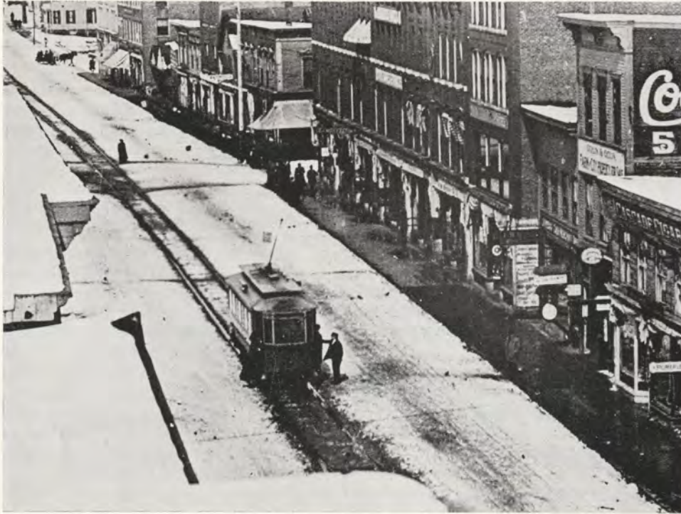
MAIN STREET, Waterville, about 1908, showing either No. 15 or 16. These two cars, both of the 20-ft. closed type, were formerly Nos. 1214 and 1215 of the Boston Elevated Railway and were purchased by the Waterville & Fairfield Railway & Light Co. in 1907.
