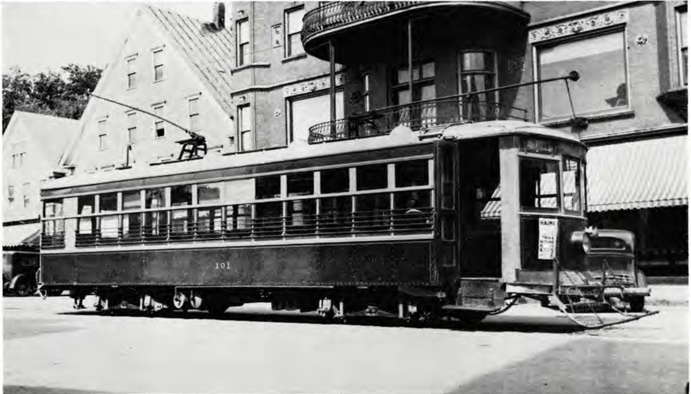
MODERN ROLLING STOCK of the Waterville, Fairfield & Oakland Railway Company was represented by this Wason-built (1922) double truck safety car, acquired along with Nos. 102 and 103 from the Rockland, Thomaston & Camden Street Railway Company in 1931. Photograph was taken at Fairfield, June 18, 1935, by Roger Borrup.
