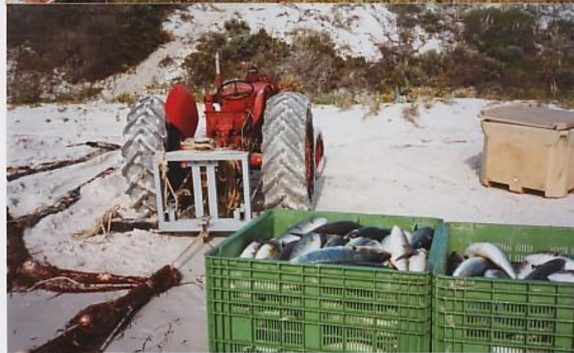
Red tractor, with rear mounted capstan winch. Two 0.5t bins, ice bin.
