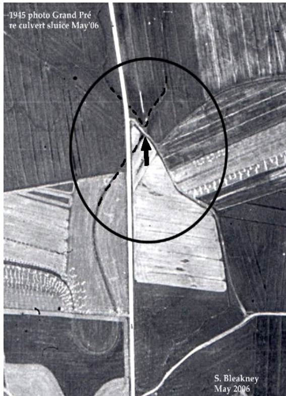
FIGURE 5: The roadway (white line) under which the sluice was discovered as seen from the air in 1945. The black arrow indicates the find location at the point where the road crosses the creek bed (the course of the creek is indicated by dashed lines). North at top. SOURCE: Sherman Bleakney (A8645-53, 1945). ©Department of Natural Resources Canada. All rights reserved.
