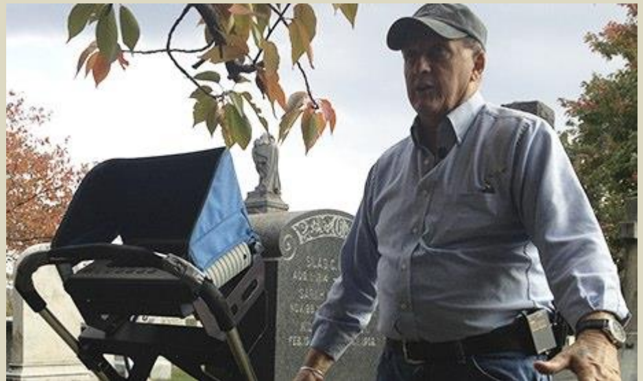
Bob Perry demonstrates ground-penetrating radar at the Historic Congressional Cemetery in Washington Leah Binkovitz
