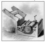
He spent the next few months building a prototype. The gin itself comprised a rotating drum with wire hooks or ratchet-like teeth that pulled cotton fibers between the teeth of a comb. The comb had teeth spaced too closely for seeds to pass through. A
